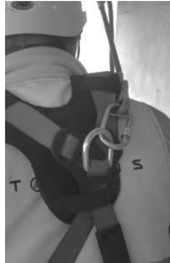
Terminal point B 25kN rated karabiner for Harness connections.
