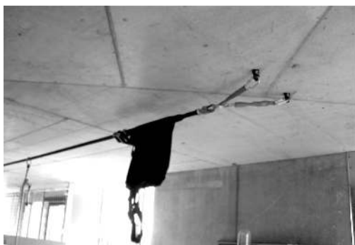
This is how the Lifeline will look when anchored and tensioned at the storage bag end.
